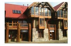
5. It is highly encouraged that awnings, deep roof overhangs or colonnades be incorporated into buildings in order to provide weather protection along sidewalks and at building entrances. These devices must be an integral part of the overall design;
